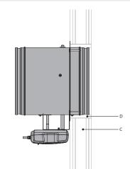
C. Light partition wall (metal studs and gypsum plasterboard) or massive wall or floor with an opening of Dn + 30 mm.D. Compressed stone wool or other approved sealing material.
